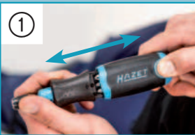
Press lock release and pull apart
