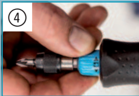
Attach screwdriver bit and lock
