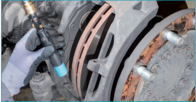
Adjustable needle carriage with integrated needle guide ensures long service life
